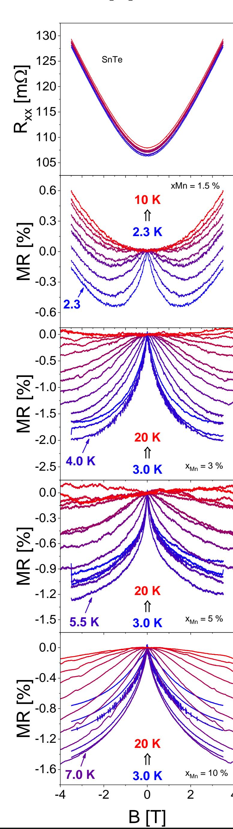
$T_c$  was determined from inverse susceptibility of AHE curves, these values agrees with the critical behavior observed on temperature dependence of  $R_{xx}$  and  $R_{xy}$
